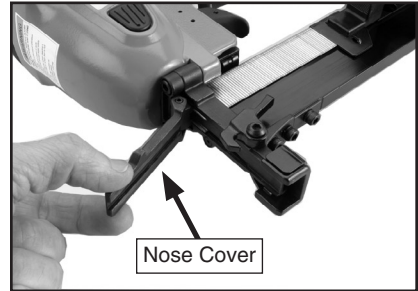
Figure 11. Opening the nose cover.
